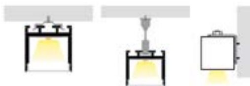
Surface-mounting, pendant or wall mounting
